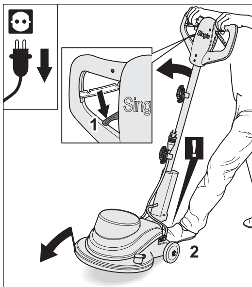
Fig. 6 Tilt the machine back up, holding it steady with your foot to stop it rolling away.
