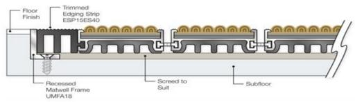
Commence installation with an unshaped mat panel wherever possible, being sure to follow the location indicated in the "Matting order confirmation form". Further panels should then be fitted, ensuring all panels are tight to the divider bars and with no gaps, except for a 1mm tolerance.
