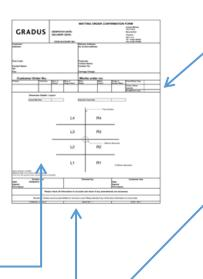
Check that each panel is clearly marked, and matches the details shown on the "Matting order confirmation form" before any installation is commenced. Where possible, prior to installation, lay the matting panels out in an adjacent clean dry area to check the panels fit together correctly and match the plan that is supplied.
